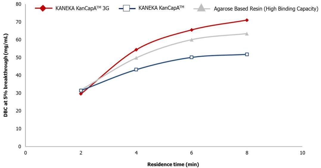
Figure 1. Dynamic binding capacity evaluation at different residence times
