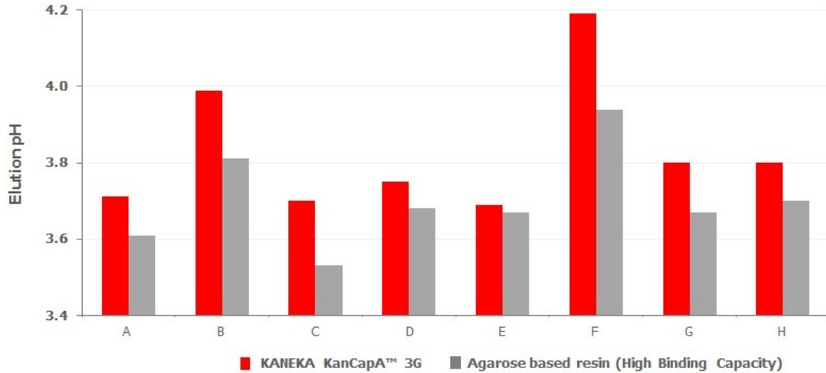
Figure 2. Elution pHs of eight antibodies from KANEKA KanCapA™ 3G compared with high binding capacity agarose based resin. Molecules A, G, H = Humanized IgG1; B, F = Human IgG2; C= Fc-fusion; D, E = Chimeric IgG. Elution pH gradient is using citrate buffer from pH 6 to 3.
