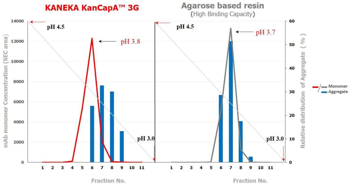
Figure 4. Aggregates separation from target mAb using a linear pH gradient elution.
